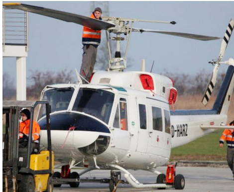
Bell 212 Main and Oil Cooler Intake Plugs
