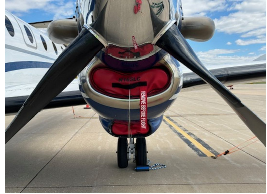
King Air Cockpit/Nose Cover, Plugs, Prop Tie/Exhaust Covers Beech 1900C ENGINE INLET PLUGS & OIL COOLER PLUGS
