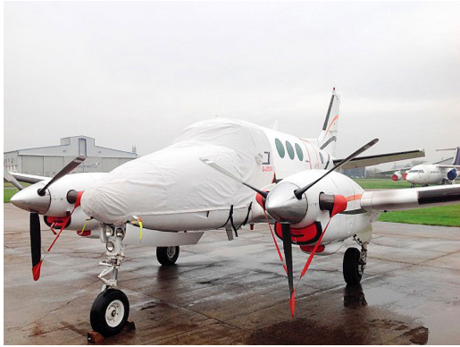
King Air Cockpit/Nose Cover, Plugs, Prop Tie/Exhaust Covers Beech 1900C ENGINE INLET PLUGS & OIL COOLER PLUGS
