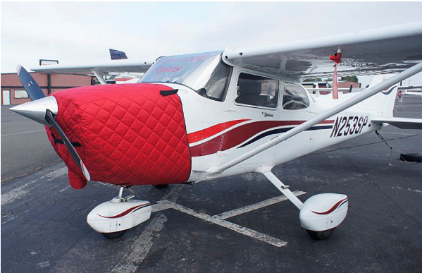
Cessna 172 Insulated Engine Cover, fully enclosed
