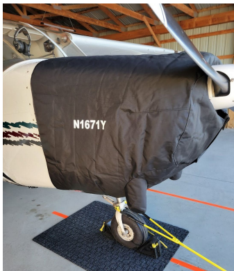
Cessna 172 Insulated Engine Cover, Fully Enclosed
